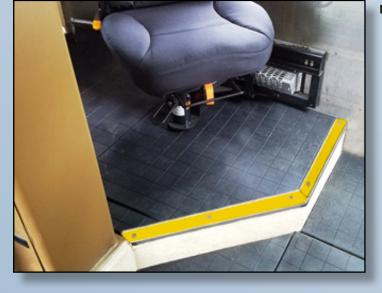
This unique Locomotive flooring, manufactured from recycled tire crumb rubber, has proven to reduce noise levels in the cab by 2 to 5 decibels after installation and has a 40% non-transmittance of vibration.
