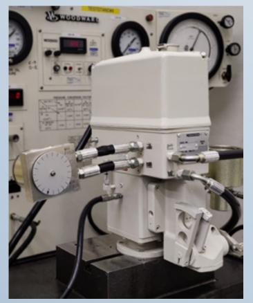
With PowerRail Governors, the highest quality standards and requirements are factory-audited, ensuring strict compliance. Only genuine Woodward parts and certified, calibrated tools and test stands are used. A complete disassembly, bench inspection, comprehensive cleaning, reassembly and testing to OEM specifications occurs with each governor to ensure Woodward requirements are met.
