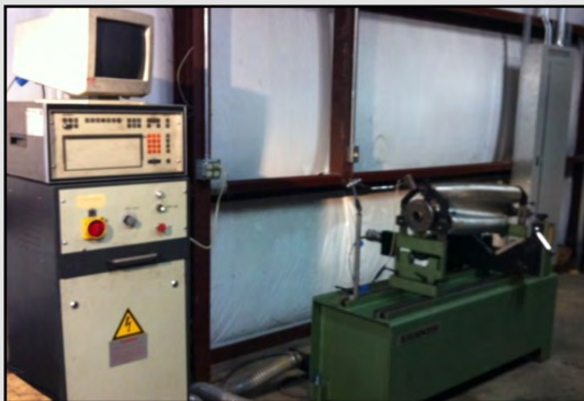
All Rebuilt Roots Blowers are Bench Tested
