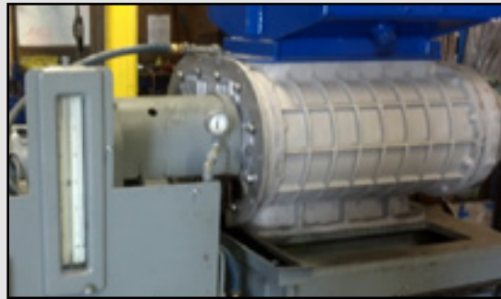
All Rebuilt Roots Blowers are Bench Tested
