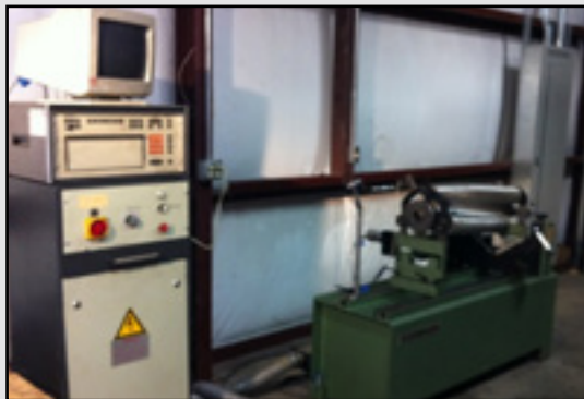
All Rebuilt Roots Blowers are Bench Tested
